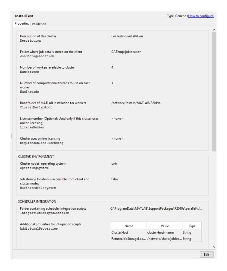
To check that the profile works, perform a validation following the steps in "Validate Cluster Profile and Installation" on page 3-48.
