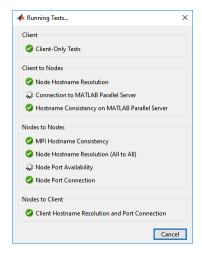
When the tests are complete, the Running Tests dialog box automatically closes, and Admin Center displays the test results in the Connectivity Testing dialog box.
