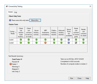
Double-click any of the symbols in the test results to drill down for more detail. Use the Log tab to see the raw data from the tests.
